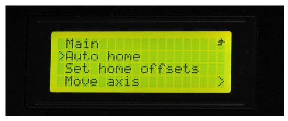
If you want to manually move the motor, you can unlock the motor. Unlocking method: Prepare>Disable steppers:
