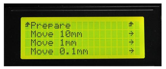
Choose the axis that you want to move by using Move X/Y/Z options. Turning the knob can make each axis move left and right or back and forth.
