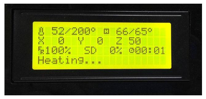
When heating is completed, it begins printing automatically.
